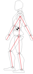
Fig. 1. Sagittal plane and joints of the robot simulation for the implementation of stability control. The red lines represent the links of the robot.
